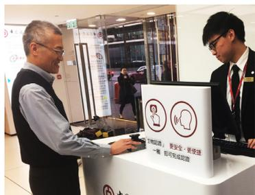
Finger Vein Authentication makes use of biometric technology to identify the unique pattern of blood flow in superficial blood vessels of the finger for customer identity verification. Finger vein pattern is unique and stable i.e. each person has different finger vein pattern and the vein pattern of each finger is non-repetitive, making it difficult to counterfeit. This helps to prevent fraud and provide protection to customers.
